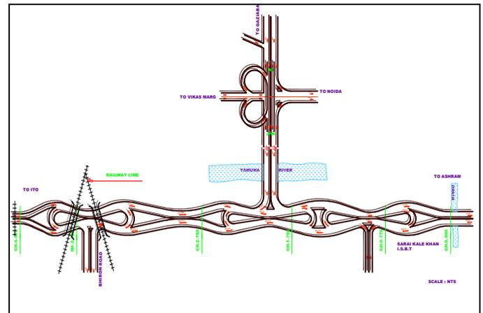
Figure 10. Integrated scheme I (loops at western approach and partial cloverleaf at eastern approach)
