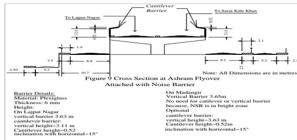
Figure 9 Cross Section of Ashram Flyover Attached with Noise Barrier
