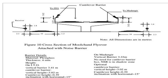
Figure 10 Cross Section of Moolchand Flyover Attached with Noise Barrier
