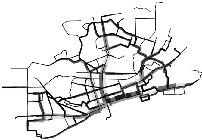
Figure 4. The diagram of distribution of volumes of transportations of the passengers on a network of city of Rostov-on-Don.
