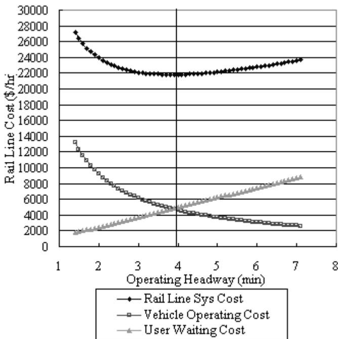
Figure 7. Costs vs. operating headway for rail line 9.
