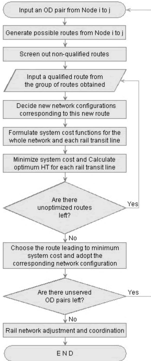
Figure 2. Flowchart for the rail network optimization algorithm.
