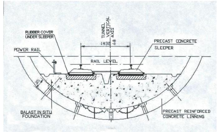
Figure 6. Reinforced concrete sleepers on concrete foundation track
