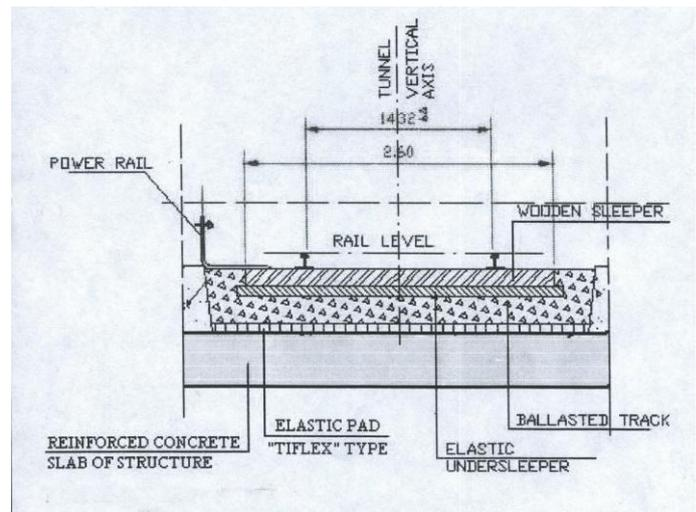
Figure 7. Ballast bed track with elastic pad
